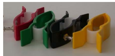
Figure 5.14 Body-surface biopotential electrodes (a) Metal-plate electrode used for application to limbs. (b) Metal-disk electrode applied with surgical tape. (c) Disposable foam-pad electrodes, often used with electrocardiographic monitoring apparatus.
